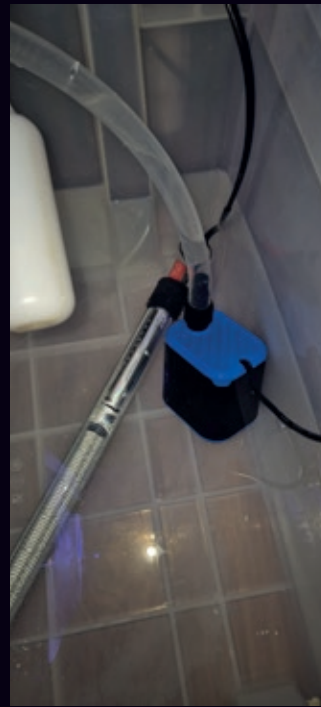
This little pump from AQQA is ideal for pumping water up out of my water mixing container into the tank. It is just the right strength to pump 25 litres over the space of 5 minutes or so... not too fast and not too slow. The speed and even on/off setting can be controlled via the inline remote.
