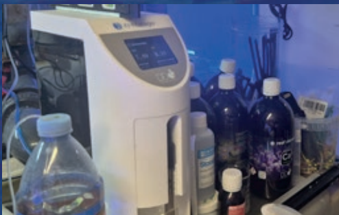
“To replenish calcium and alkalinity, David now uses Reef Zlements H2P dosing system controlled by a D-D KH/PH Manager”
