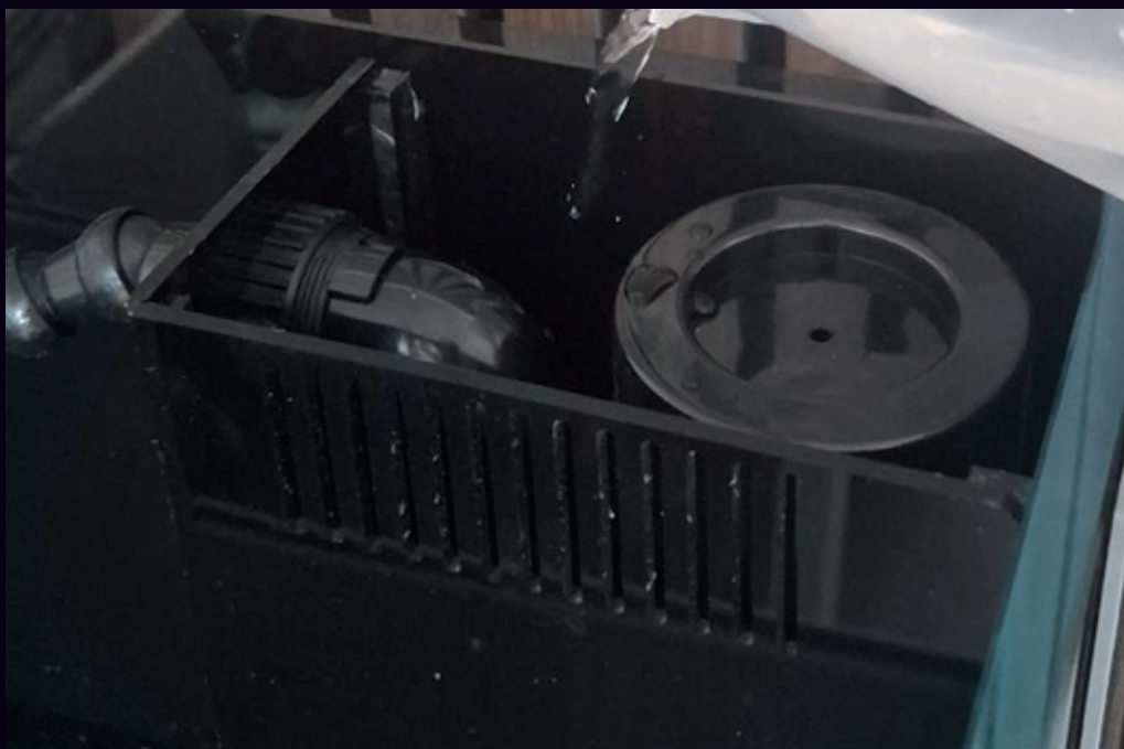
This image shows the weir box of the Clear with the lid removed (I took this pic when setting the tank up). Note that this tank only has a single overflow pipe. While this works perfectly, I often remove the silencer cap shown as it doesn't clear the water surface otherwise. With the weir cover in place there's shouldn't be any chance of anything blocking the pipe. It does make it a little noisier though.
